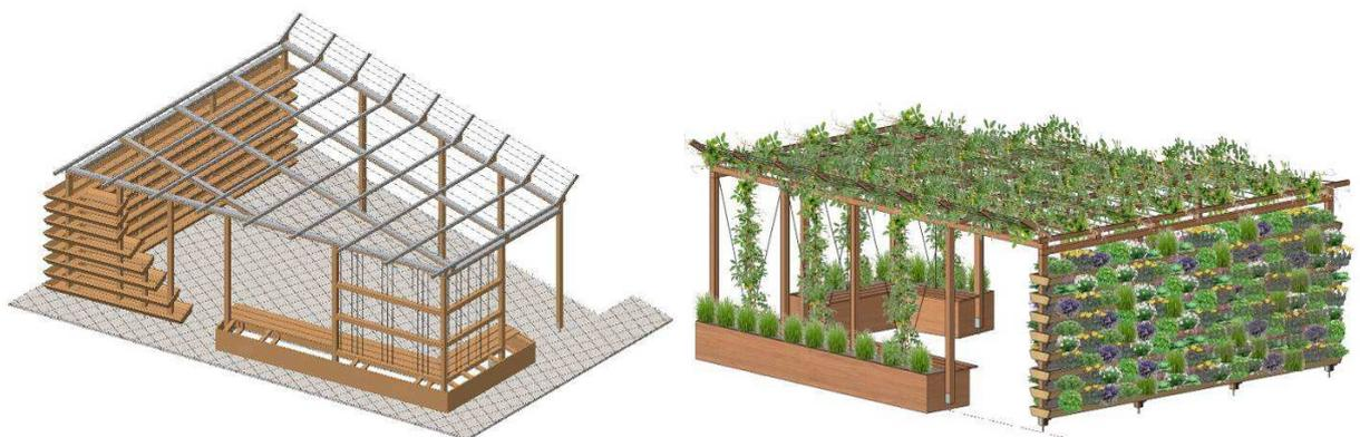
Fig. 6 and 7: Construction details and visualisation of a draft of the outdoor classroom with EVAPO+ transpiring green wall
