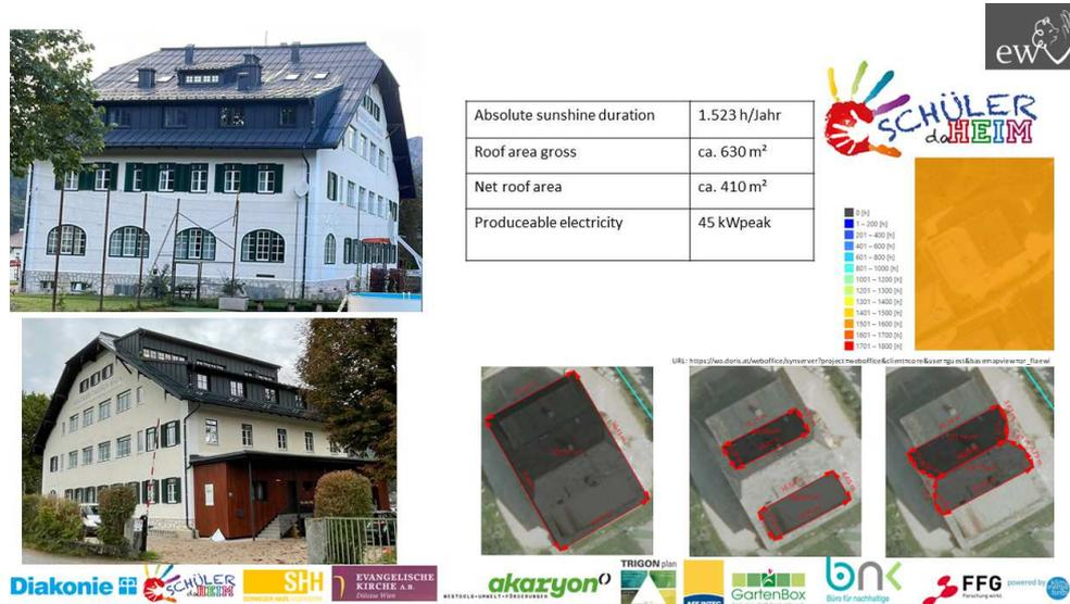
Fig. 2: Technical and Economic Pre-Dimensioning of the Photovoltaic System, Bad Goisern.
