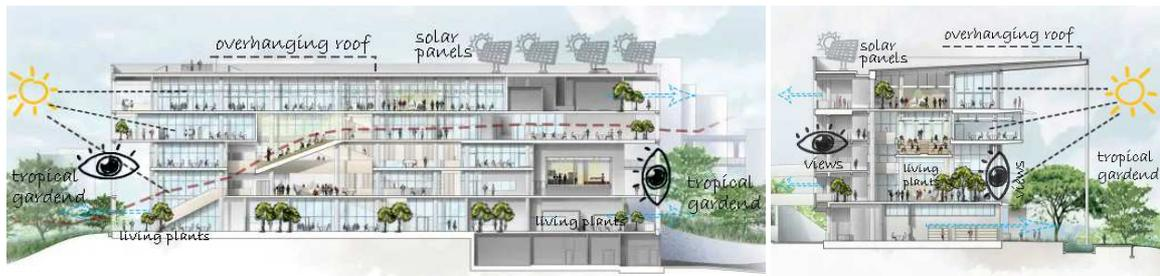
Fig. 10: Longitudinal Section components. Fig. 11: Cross Section components. Both adapted from: (“NUS School of Design & Environment”, 2022).
