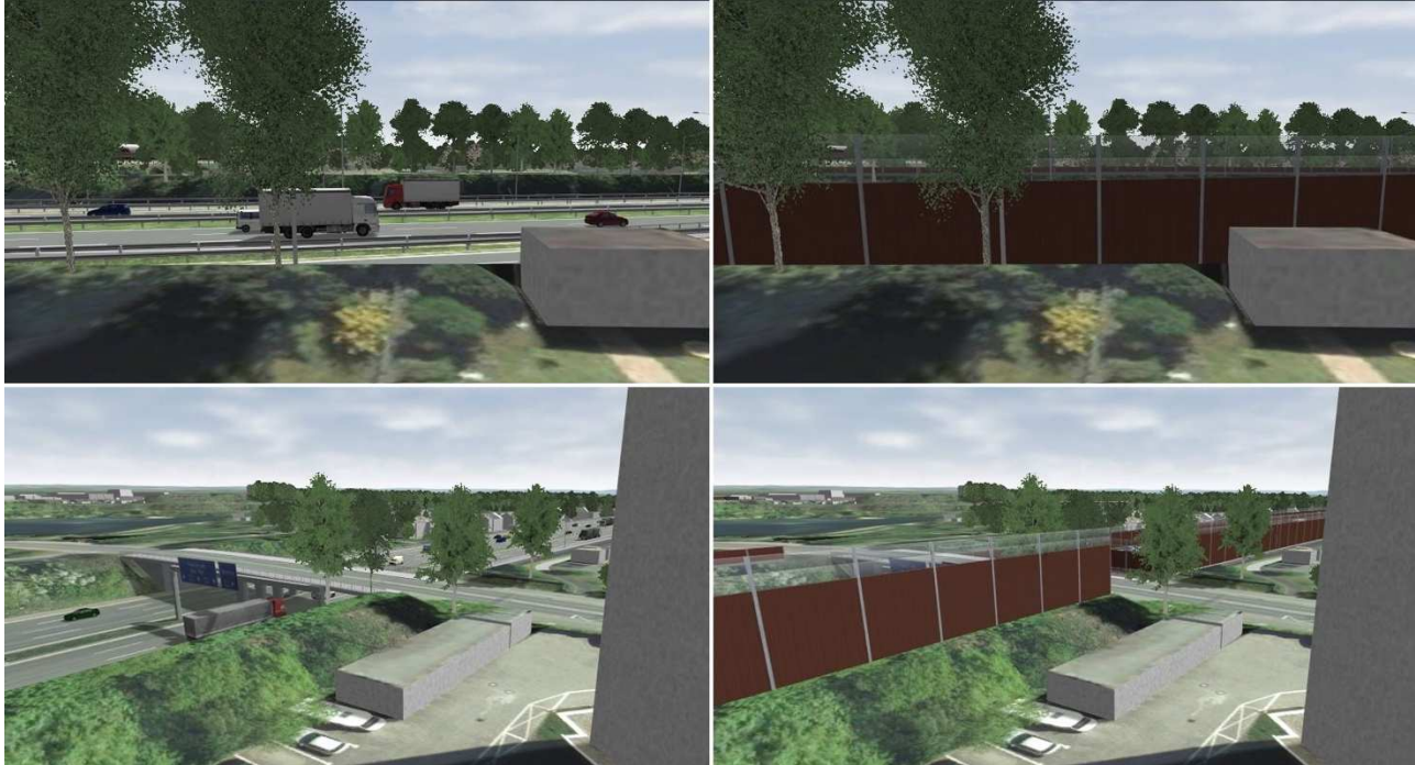
Figure 6: Inclusion of noise protection walls to address concerns of residents of the project area.
