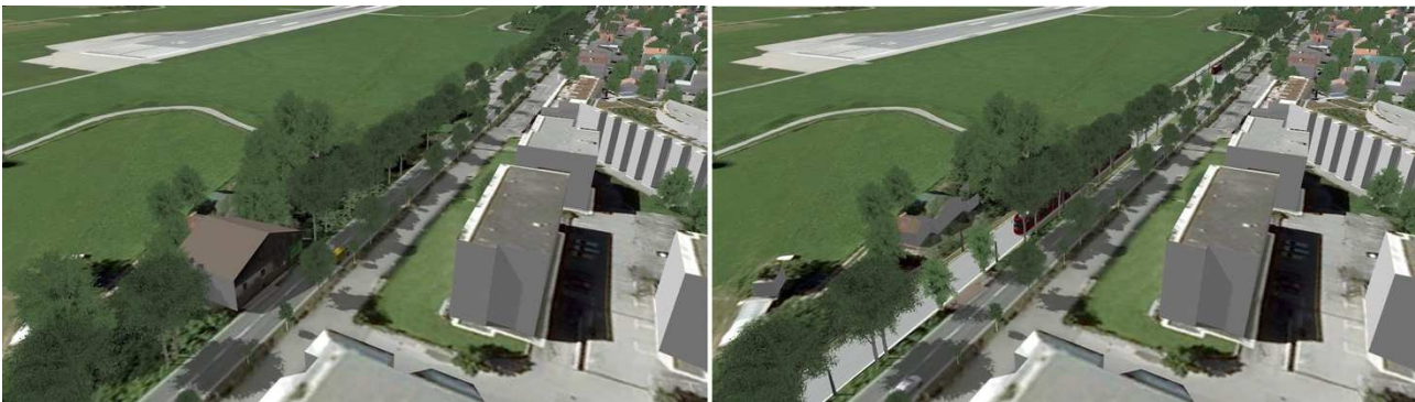
Figure 10: Addition of tramline exclusive tracks outside of the existing street by removing derelict buildings.
