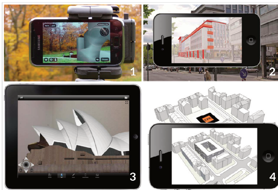
Fig. 5: AR-Software Solution: Layar POI (1) with GPS positioning, Layar Vision marker-based position recognition (2), Sightspace 3D with manual positioning via screen (3) and AR Media with local stored 3D files and marker based recognition (4). (Zeile 2017; with figures from Broschart 2013)
