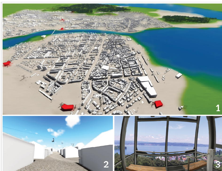
Figure 3: 3D city model of the city of Konstanz, generated in CityEngine (1) and visualized as a real-time model with planning-relevant content in Lumion (2), mixed reality film from a car (3) (BUSCHLINGER et al 2016).
