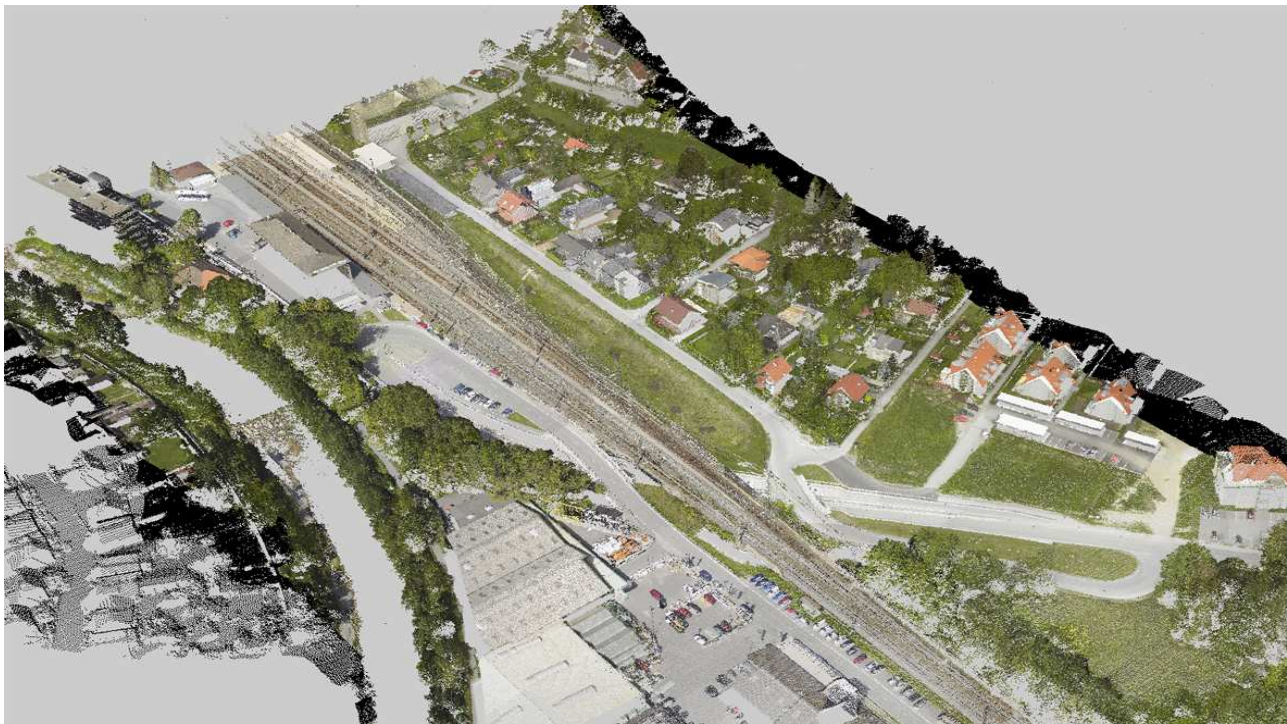
Figure 3: Laser scan data colored by orthophotography.
