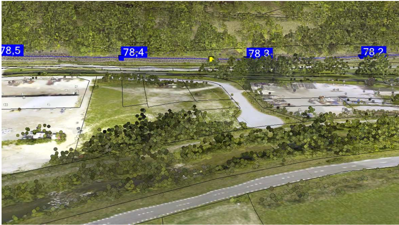
Figure 5: Close-up view. In addition to the terrain and vegetation data, GIS meta-information depicts property boundaries and railway chainage labels (in kilometers).
