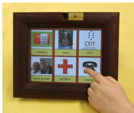
Fig. 3: Pilot study “interactive picture frame” – evaluation of user acceptance of touch screen based easy to use phone system (ordered by TELEKOM AUSTRIA)
