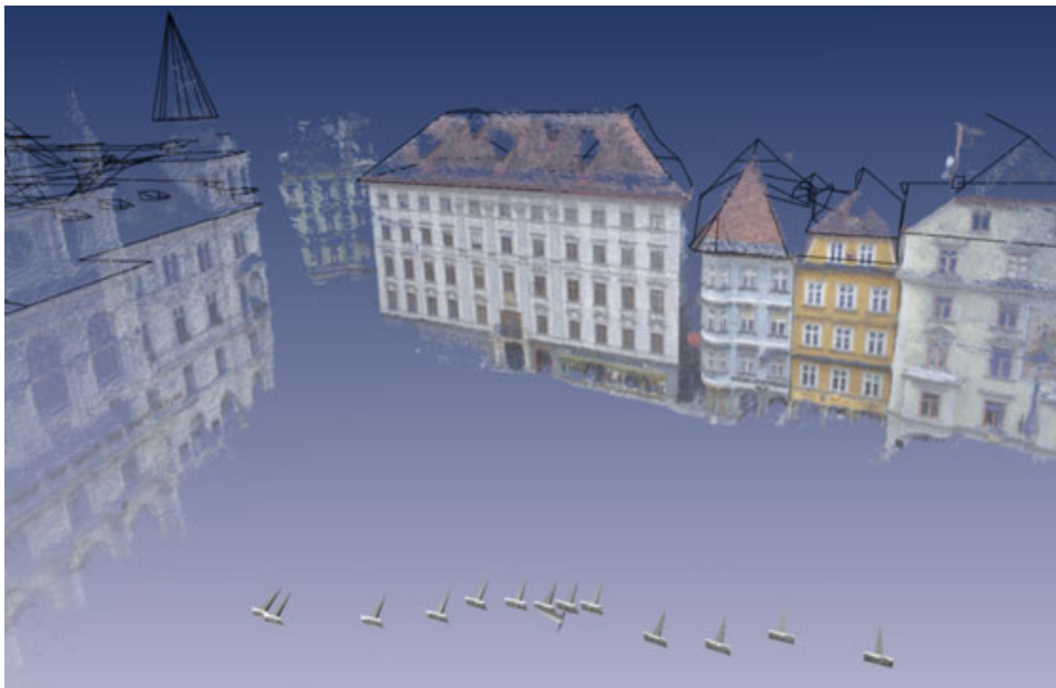
Figure 7: Two compounded geo-referenced sequences of the Grazer Hauptplatz augmented with roof lines.
