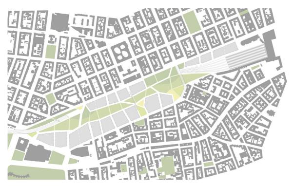
Fig. 10: Site Plan, the Block size provides frequent route choice, park provides cooling © S. Tobisch 2021
