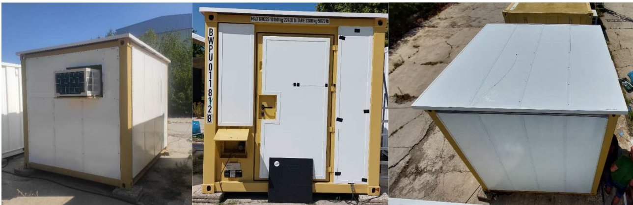
Figure 5: Container equipped with phase change composite panels at the Erding site
