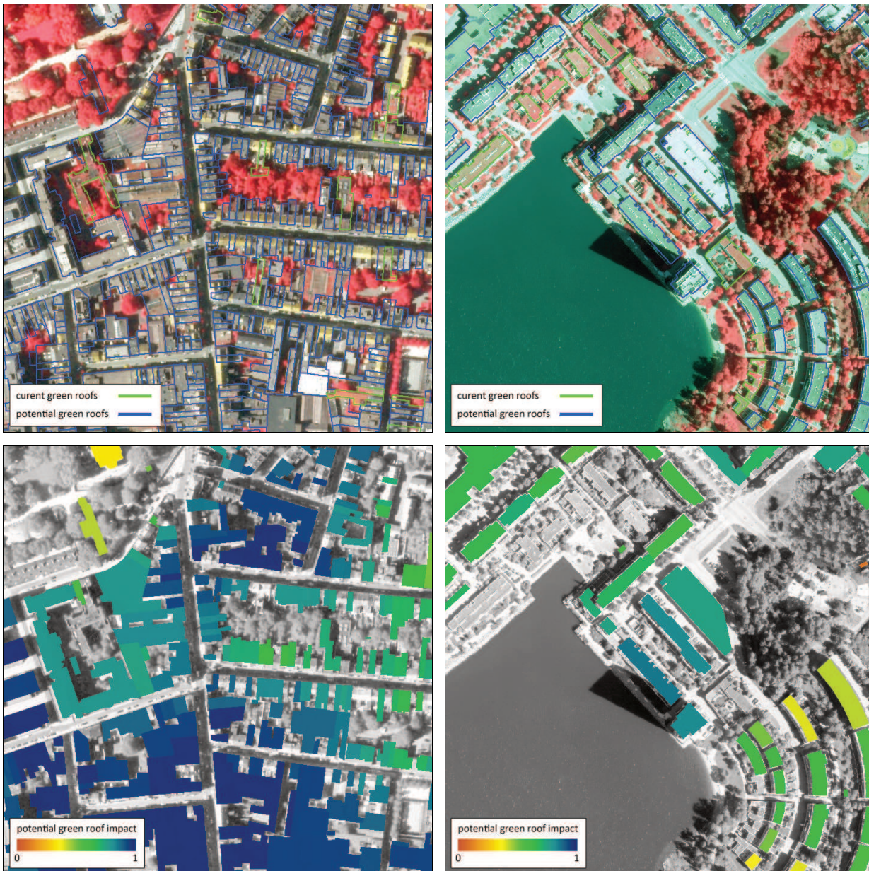
Fig. 2: Current and potential green roof maps obtained with the presented technique overlaid to the available CIR airborne imagery for a subset of the Antwerp (top left) and Helsinki (top right) study areas, along with the corresponding potential green roof impact maps (bottom left) and (bottom right), respectively.
