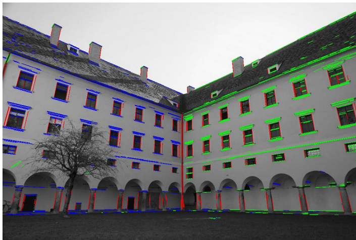
Figure 2: Detected line segments by the advanced line extraction where lines with the same color belong to the same vanishing point.
